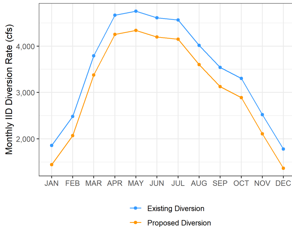
FIGURE H1-1. ESTIMATED EXISTING CONDITIONS AND PROPOSED ACTION COLORADO RIVER MONTHLY USBR DIVERSION RATES (CFS) TO IID
